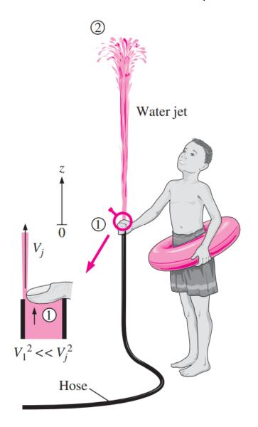
$$\frac{P_{1}}{\rho g} + \frac{V_{1}^{2}}{2g} + z_{1}^{\approx 0} = \frac{P_{2}}{\rho g} + \frac{V_{2}^{2}}{2g} + z_{2} \rightarrow \frac{P_{1}}{\rho g} = \frac{P_{\text{atm}}}{\rho g} + z_{2}$$
