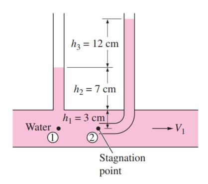
$$\frac{P_1}{\rho g} + \frac{V_1^2}{2g} + \not z_1 = \frac{P_2}{\rho g} + \frac{V_2^2}{2g} + \not z_2 \qquad \rightarrow \qquad \frac{V_1^2}{2g} = \frac{P_2 - P_1}{\rho g}$$
